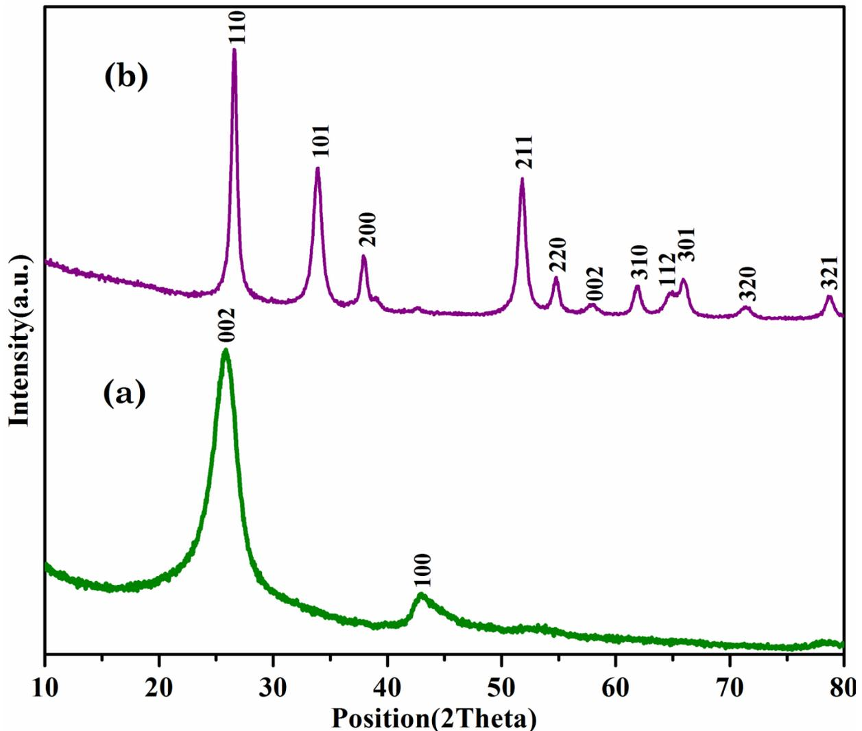
Figure 3 XRD patterns of (a) as received MWCNTs (b) SnO<sub>2</sub>/CNT nanocomposites
