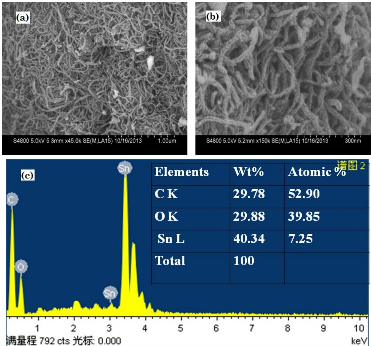
Figure 2 FESEM images of (a,b) SnO<sub>2</sub>/CNTs composites and (c) its EDX
