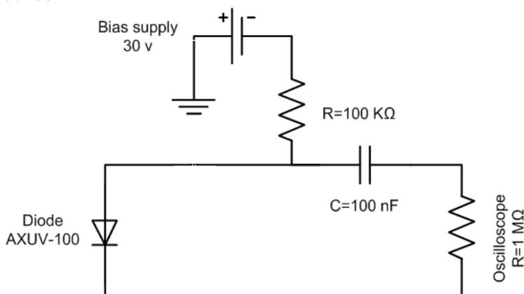
Figure 5 Scheme for reverse biased operation of the AXUV-100 photodiode.
