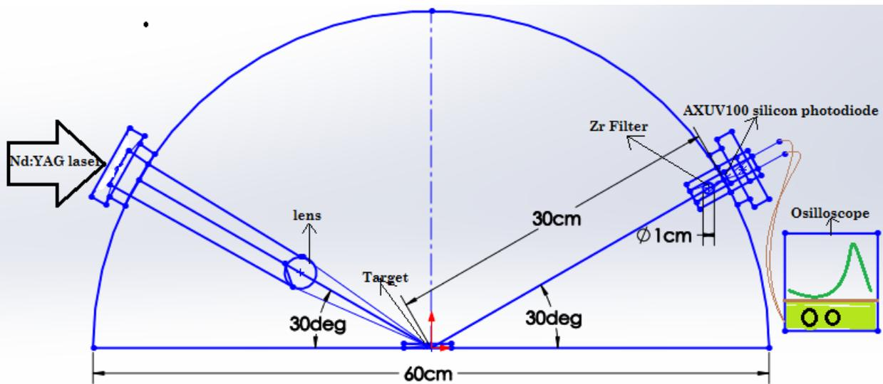
Figure 1 schematic of Experimental setup for EUV source
