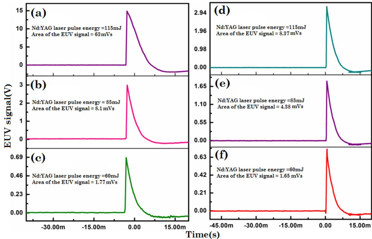
Figure 6 AXUV100 photodiode response for laser pulse energy (a-c) for pure Sn and (d-f) for SnO<sub>2</sub>/CNTs nanocomposites.
