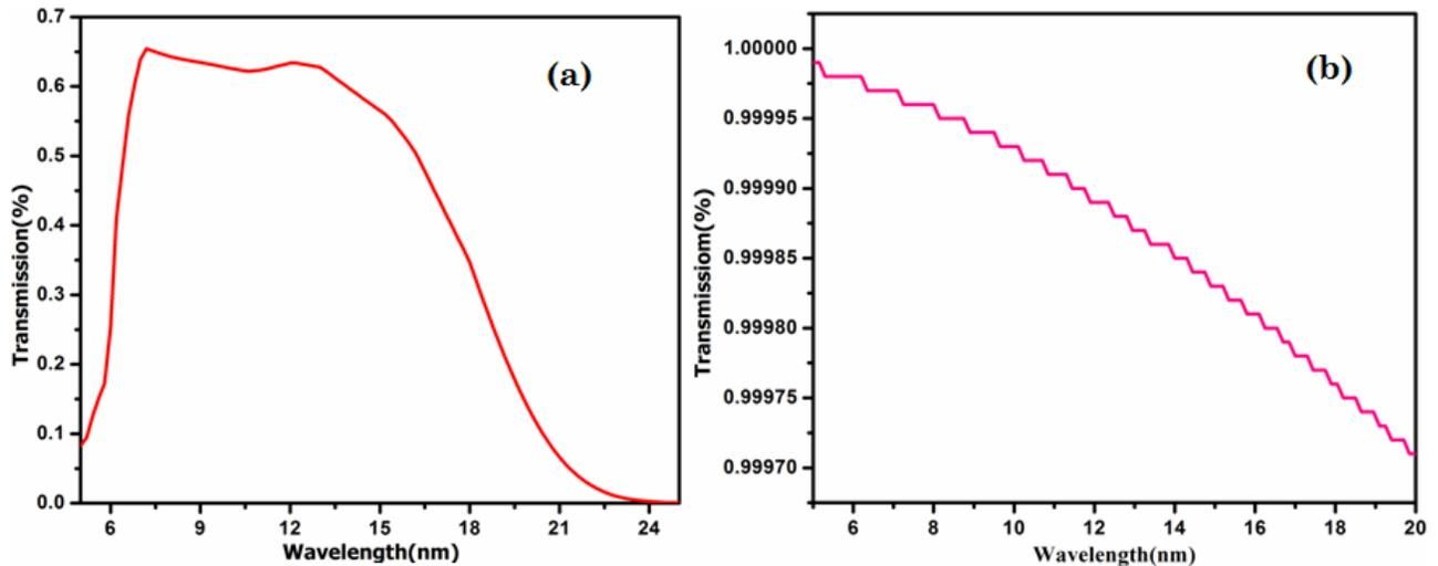
Figure 4 Transmission spectrum for (a) solid (Zr filter, 140nm thickness) and (b) gas (with chamber pressure of  $5.5 \times 10^{-5}$  torr) for EUV radiation
