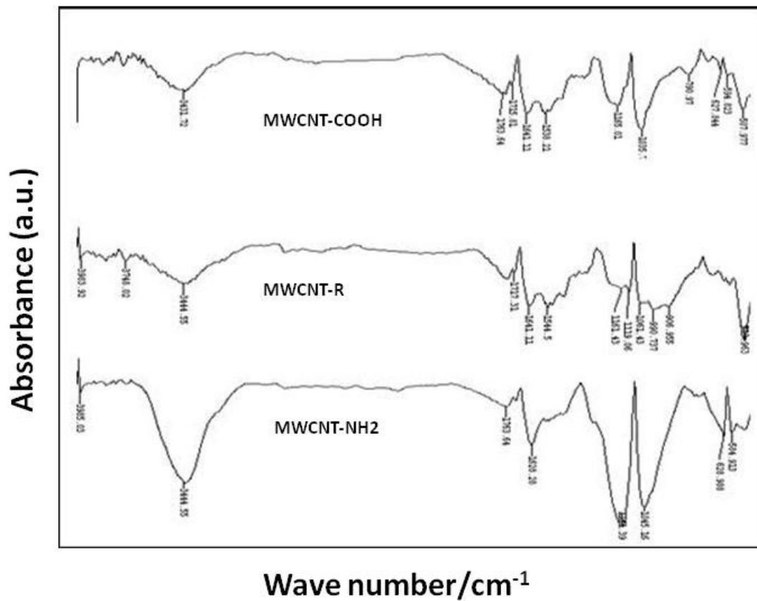
Fig. 1. FTIR spectra of functionalized MWCNTs.
